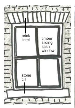
Simple but well detailed Victorian window surround with a contrasting brick lintel and stone window cill
